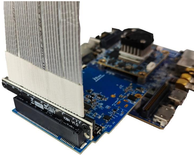
Figure 19: PCIe x8 Cable insertion into FMC Module
